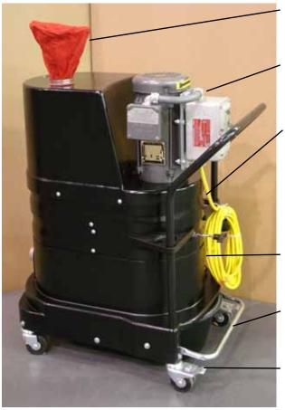
*Air Diffuser/Silencer:* The exhausted air from the turbine is diffused to prevent the re-entrainment of laden dust. The motor deck silencer provides a quiet working environment, even in continuous use.
